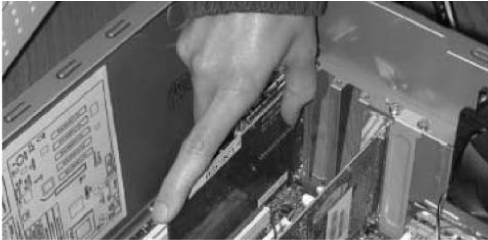
Figure 2.1: Inserting the DVD board into PCI slot
